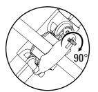
Turn the knob clockwise to completely tighten the rear clamp.
