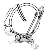
Turn the knob clockwise to tighten hoop.
