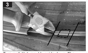
Turn roof ditch mould upside down. The underside rib has metal inside. Use side cutters to cut either side of hole position.
