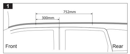
Roof ditch moulding requires holes to expose the roof rack fixing points. Mark points at measurements shown above.
