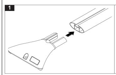
Insert the sports leg fully into the cross bars, a rubber mallet may be required to knock the leg in place.
