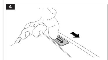
Locate the cover plates on the roof channel trim. Slide the cover plates in the direction of the arrow to remove. This exposes the M6 threaded boss.
