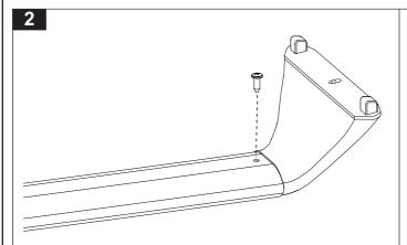
From the underside of the cross bar insert the phillips head screw.
