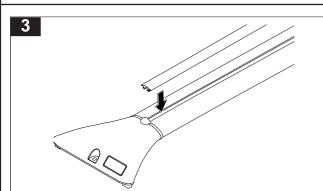
Insert the correct rubber buffer strip into the top of the cross bar.
