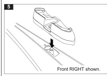
Place the correct roof pad over the M6 threaded boss in the roof channel. The pads are marked on the underside with part numbers to denote their position on the roof. There is also an arrow on each pad which must point forward once installed.
