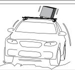
**WARNING! Important Load Carrying Instructions** With utility vehicles, the cabin and the canopy move independently. Roofracks and vehicle can be damaged if the item transported is rigidly fixed at points on both the cabin and canopy. Instead, rigidly fix to either the cabin roofracks or the canopy roofracks.
