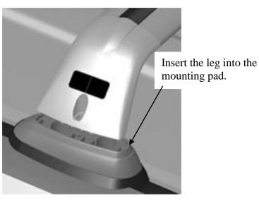
11: Insert the support leg assemblies into the mounting pads. The crossbars are identified as Front, Middle and Rear, refer the crossbar layout.
