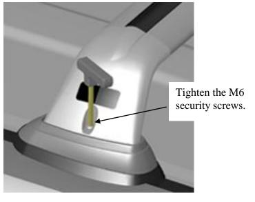
**14:** Using the security Allen key provided tighten support leg attachment screws to secure the crossbars.
