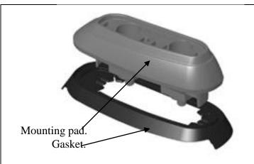
**8:** The mounting pad gaskets are identified L & R. The L gaskets fit the left side pads, the R gaskets the right side gaskets. The direction arrows on the pads and gaskets must face the same direction.
