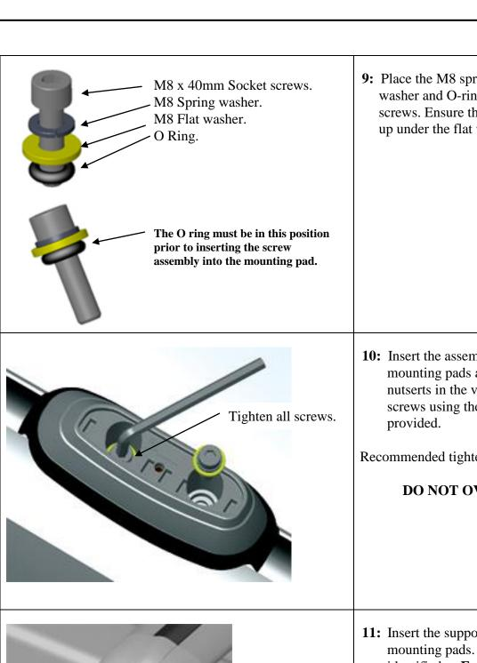
**9:** Place the M8 spring washer, M8 flat washer and O-ring onto M8 x 40mm screws. Ensure that the O-ring is pushed up under the flat washer.
