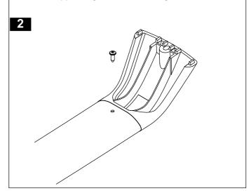
Determine the required crossbar positions as per the crossbar information on page 1. Remove the trim screws using the 4mm Allen key provided. Store the screws in a safe place for refitting if the crossbar mounting pads are removed.
