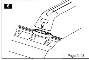
Place the M6 spring washer and M6 flat washer onto the M6 security screw. Insert the screw assembly into the leg and screw into the roof.
