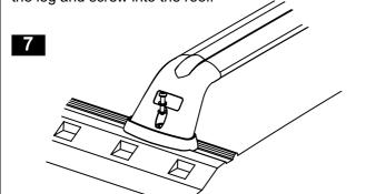
Tighten the M6 crossbar attachment screw to 5Nm using the security Allen key provided. Do not over tighten.
