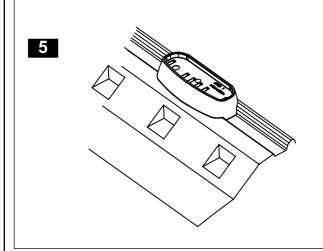
Place the pre-assembled crossbar assembles onto the mounting pads. The crossbars are marked **Front** and **Rear**. Front on the front of the vehicle, Rear on the rear of the vehicle.
