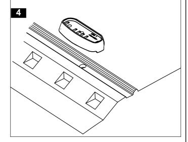
Check that the mounting pad is aligned with the hole.
