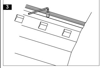
Place the mounting pad onto the roof, locating the hole alignment boss in the trim screw hole.
