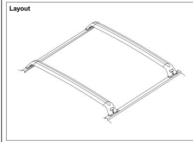
Remove the four covers from the roof rack mounting locations by carefully inserting a small bladed screwdriver into the cut outs in the rear of the cover and lever upwards carefully.
