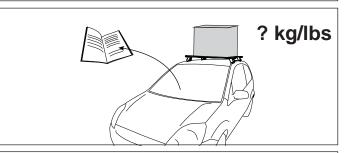
When these roof racks are to be used on a vehicle that is driven off sealed roads, the manufacturer maximum roof load rating (found in the vehicles User Manual) should be divided by 1.5. Subtract 5kg/11lbs from your maximum carrying capacity to account for the weight of the roof racks.
