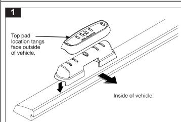
The four top and bottom pads are identical. Diagram at left shows correct orientation of top and bottom pad . The large cut out and lip of the bottom pad sits over the inside edge of the roof rail.
