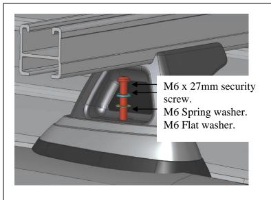
13: Place the M6 spring washer and M6 flat washer onto the M6 x 27mm security screw. Insert the M6 screw assemble through the heavy duty leg and screw into the mounting pad.
