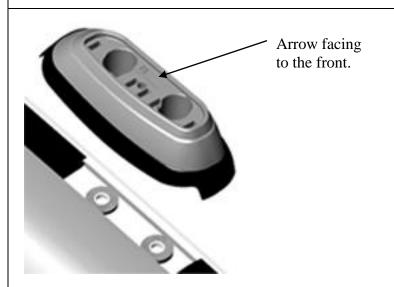
**9:** Using the mounting pad layout as a guide, place the pads onto there respective positions. **Note:**
