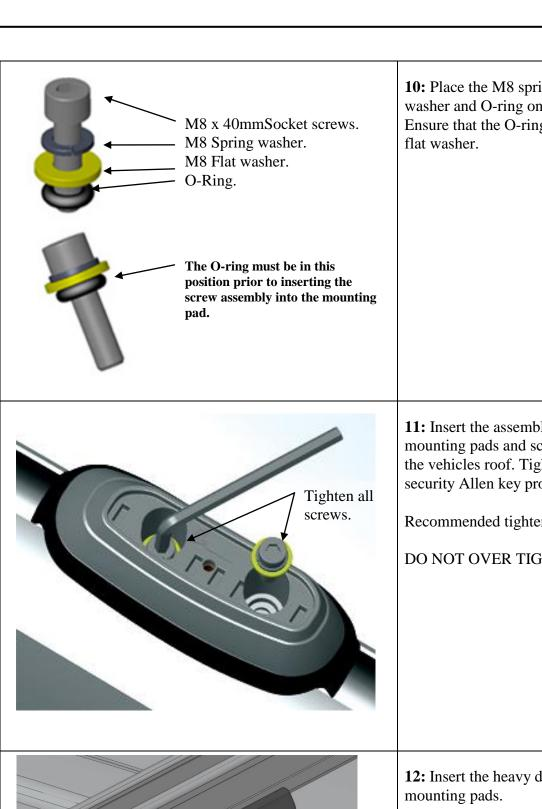
**10:** Place the M8 spring washer, M8 flat washer and O-ring onto M8 socket screws. Ensure that the O-ring is pushed up under the
