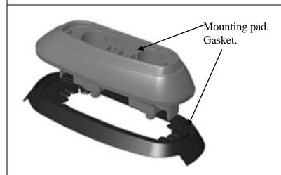
**8:** The mounting pad gaskets are identified L & R. The L gaskets fit the left side pads, the R gaskets fit the right side pads. The direction arrows on the pads and gaskets must face the same direction.
