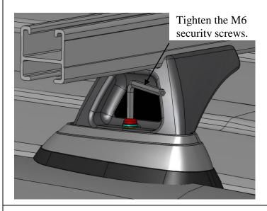
Using the security Allen key provided tighten heavy duty leg attachment screws to secure the crossbars.
