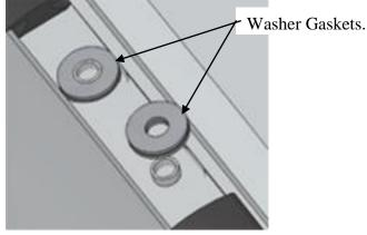
**4:** Place the gasket washer onto the plastic tube attachment bolt locators in the vehicles roof .
