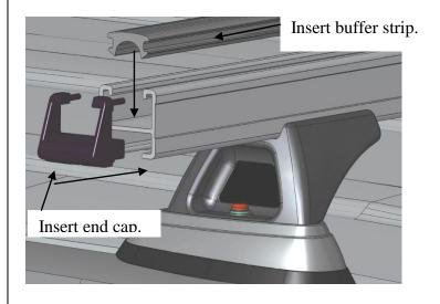
**17:** Insert the crossbar rubber buffer strip into the top of the bar.
