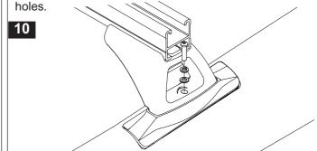
Using the allen key provided, tighten the support leg screws to secure the crossbars. Recommended tightening torque 4N/m. DO NOT OVER TIGHTEN.
