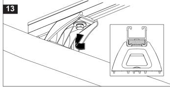
Insert the crossbar rubber buffer strip into the top of the crossbar. Insert the end caps into the ends of the crossbar, a rubber mallet may be required to fit the end
