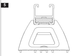
Each mounting pad is identified with a pad position and part number. The mounting pad positions are, front left, front right, rear left and rear right side pad. Note: The right hand side of the vehicle is the driver side.
