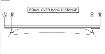
Tighten the crossbar attachment bolts. Recommended tightening torque 5N/m. DO NOT OVER TIGHTEN. Check that the channel nut is located across the crossbar.
