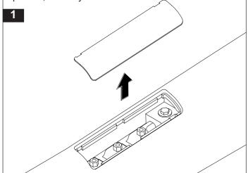
Using a M6 x 27mm screw and allen key provided, screw the screw into the each of the mounting nutserts, as shown in the diagram below, to clean out the threads. Care should be taken not to damage the paint under the nutsert.
