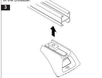
Tighten the leg attachment bolt so that the channel nut turns to locate across the crossbar. Finger tighten the bolt, as the legs will require adjustment later.
