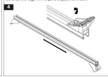
Check that the channel nut is fully located across the bar.
