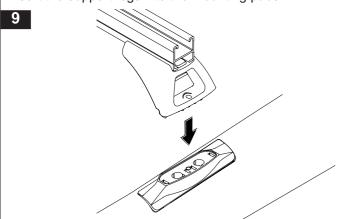
Assemble the M6 spring washers and flat washers onto the M6 x 27mm security screws. Slide the crossbar across to give access to the attachment screw hole. Insert the screw assembly into the support leg mounting holes.
