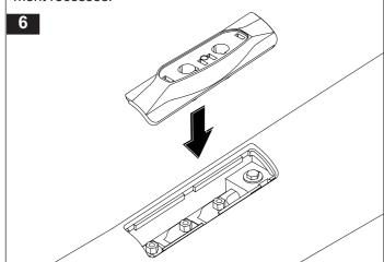
Assemble the M6 spring washers and flat washers onto the M6 x 16mm security screws. Insert the screws into the pad mounting holes and using the allen key provided carefully tighten. Recommended tightening torque 4N/m. DO NOT OVERTIGHTEN. Repeat this process for each pad.
