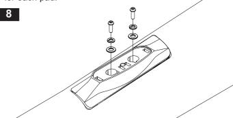
Insert the support legs into the mounting pads.
