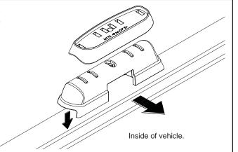
Place the base pads on the roof rail at 290mm from the front join on the roof rail then 605mm between the pads.
