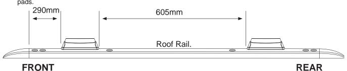
Place your crossbars onto the pads. Place the stainless strap into the inside gap of the base pad. Insert the M6 x 40 bolt and washer assembly through the leg and fasten. **Recheck measurements from step 2 and tighten**
