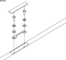
Each mounting pad is identified with a part number, position code and direction arrow. The arrow must point toward the front of the vehicle. The mounting pad position codes are as follows:
