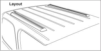
Using a pencil mark out a drilling centreline **60mm** from the edge of the 2nd roof channel in. Use one edge of the Track as a straight edge to rule a line (this will be the centreline of the Track). Using a Tape Measure plot 5 points taking each measurement from the small groove towards the rear of the canopy. Measure 85mm from that same groove and place a line, this is where the end of the track will lie.
