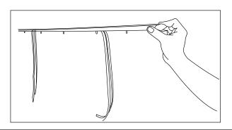
Align each T-bolt so that it drops into its corresponding hole position. The end of the track (not the end cap) must lie **85mm** from the groove towards the rear of the canopy.
