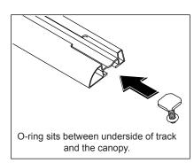
Insert the End caps into each end of the track. Peel the backing tape off the underside of the track.
