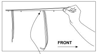
4 Door: 1 off M6 x 45mm Sq head bolt per side, second hole from front.
