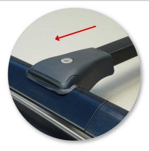
Pull legs out evenly until both rubber gasket seal on roof rail.
