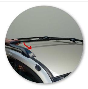
Place one end of the crossbar on the opposite rail then swing the leg assembly closest to you onto the rail into the original position.
