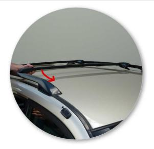
Place one end of the crossbar on the opposite rail then swing the leg assembly closest to you onto the rail into the original position.
