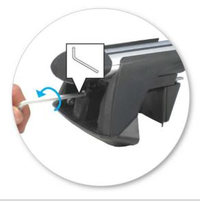
Use 5mm Hex Key to loosen locking screw and open clamp.
