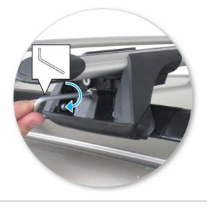
Use 5mm Hex Key to tighten clamp and secure crossbar to rail.
