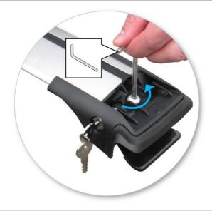
Using Hex Key, reverse the leg screw 10 turns.
