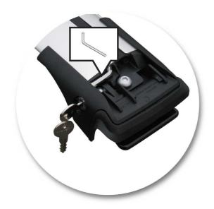
Locate the Hex Key in one of the roof rack legs.
