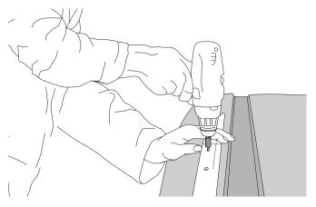
NOTE: A drill stop is used to avoid drilling into the second roof skin of the vehicle.
