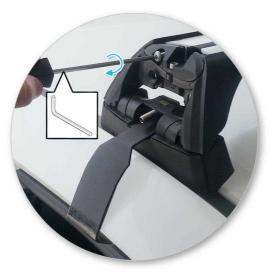
Tighten adjusting screw to 2 Nm (1.5 ft lb) hand tight.
