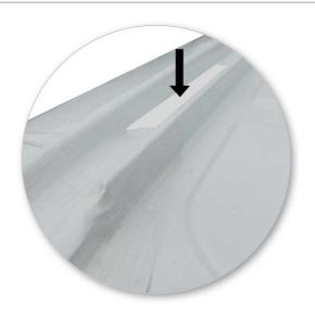
Apply masking tape to vehicle roof in all positions.
