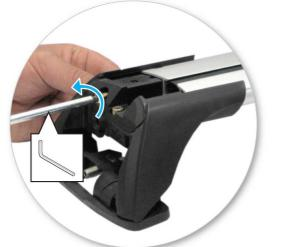
Use hex screwdriver to reverse adjusting screw 10 turns.
