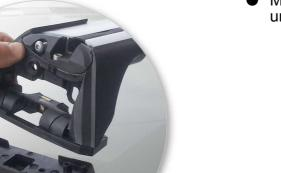
• Make sure the pad fits into the holes underneath the foot.
