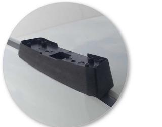
Place rubber pads (supplied with fitting kit) on the vehicle roof. Pad may vary in shape to that shown.
