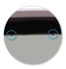
• Locate vehicle fixed point for the rear bar as indicated on rear window.
