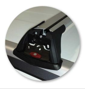
Ensure the plastic knob is in the position shown when fully tightened.
