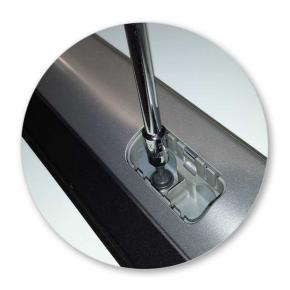
Remove screws from the vehicle's fixed points
