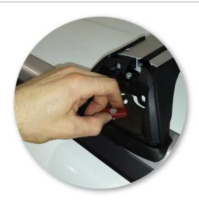
Using the bolts with plastic knobs, attach crossbars to the nuts by fitting the bolt through the internal block on the foot and screwing it into the nut.
