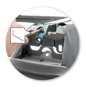
Tighten adjusting screw to 3 Nm (2.2 ft lb) hand tight.
