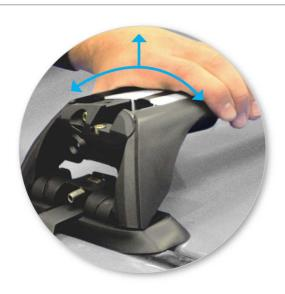
Check crossbar is securely attached to the vehicle.
