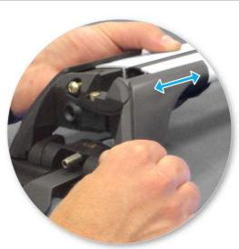
Adjust the legs on the crossbar so that they are positioned equally from the ends of the crossbar, and the clamps engage firmly on the body work of the vehicle.
