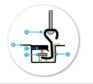
A= Clamp B= Roof line C= Body trim D= Vehicle fixpoint E= Protective strip
