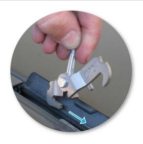
Hook small claw into rear of the clamping block
