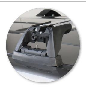
Ensure the pads are in the correct position and the clamp threads pass through the crossbar feet.
