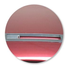
Open fixed point cover by sliding with downwards pressure.
