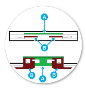
Ensure part B is engaged under mounting point and part A is behind the mounting point.
