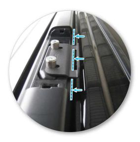
• Ensure edge of rail aligns with edge of slot.
