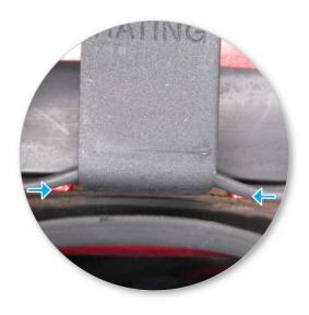
When viewed from the top, clamp should be lined up with the two lugs on both sides.
