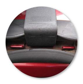
• Insert clamp into the mounting point.
