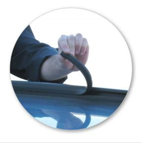
Locate and remove rubber seal from inside edge of roof rail on vehicle.
