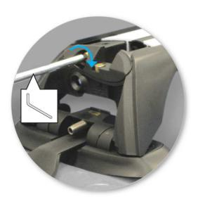
• Tighten adjusting screw to 5 Nm (3.7 ft lb) hand tight.
