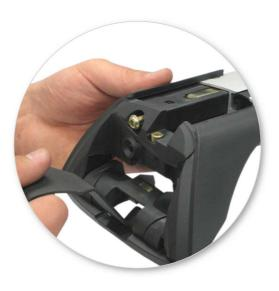
Attach clamp to each leg. NOTE; clamps may have labels showing their positions on the vehicle (For example; "Front Right").
