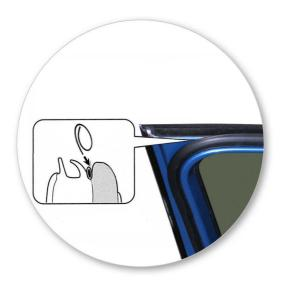
Ensure door seal positioned as shown.
