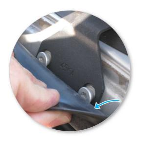
Locate vehicle's fixed points behind door frame rubber.
