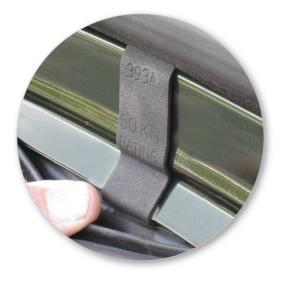
Pull down rubber and slide body clip up and over the interior trim. Refit the rubber over the clip.
