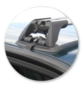
• Refit rubber seal over the clamp.
