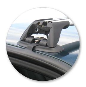
• Refit rubber seal over the clamp.
