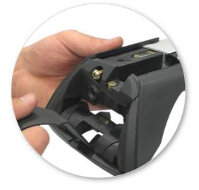
Attach clamp to each leg. NOTE; clamps may have labels showing their positions on the vehicle (For example; "Front Right").
