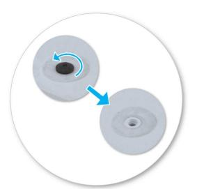
Remove fixed-point cover screws with 5mm Hex Key.
