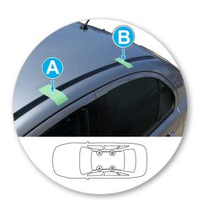
Apply masking tape to ditch in all four positions.
