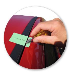
• Carefully remove centre section of ditch mould with flat-head screwdriver.
