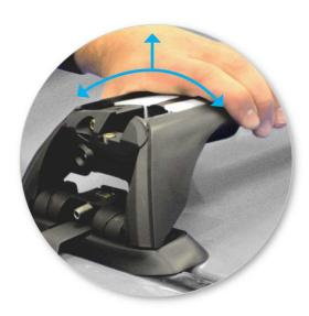
Check crossbar is securely attached to the vehicle.
